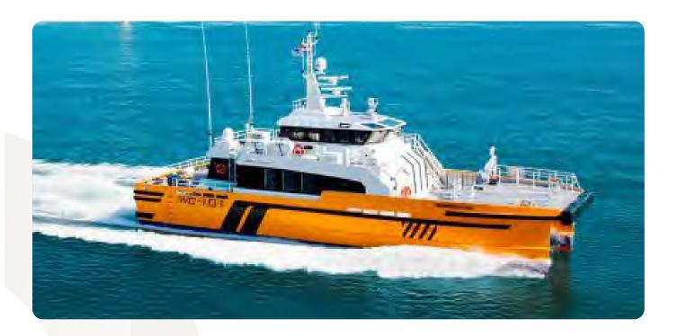
These types of boats are out on open sea, and thus should be able to manoeuvre well in high waves, strong winds and currents. Typically, they are out 12 hours a day (3000-4000 operations per year). For most of the time they travel at 30 knots (high speed).
